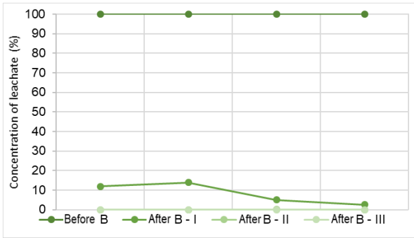
Fig. 8 - Chart of concentration of leachate during time in test B
